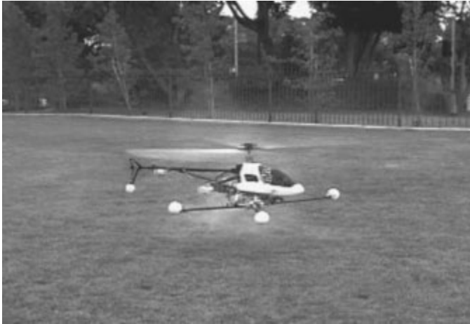
Fig. 6.1.13. Dr. Jim Montgomery, University of Southern California Robotics Research Laboratory. Autonomous Vehicle Aerial Tracking and Retrieval (AVATAR) project. A flying robot uses sensors and loosely coupled computing modules to intelligently control its own flight, ( http://www-robotics.usc.edu/~avatar/ ).
