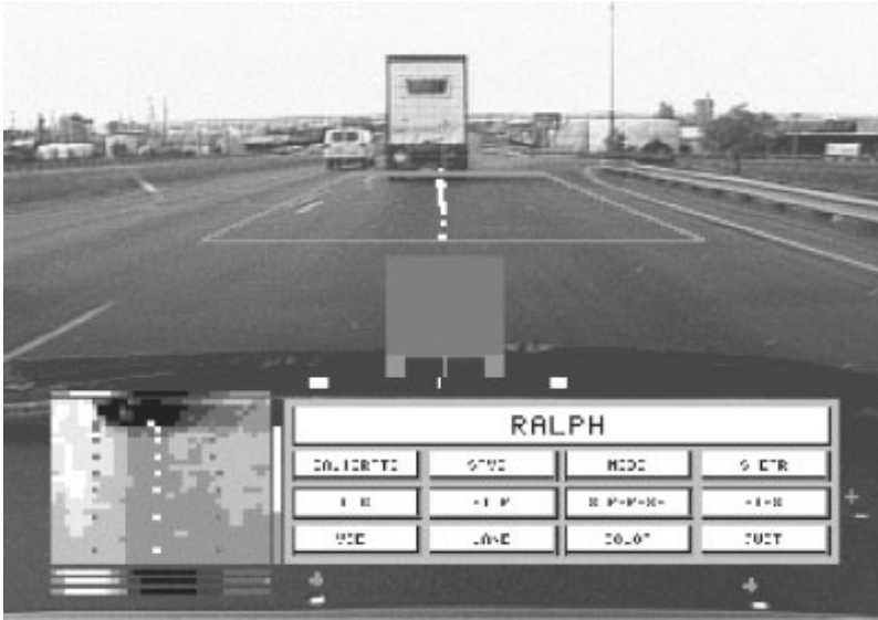
Fig. 5.1.4. No Hands across America Project (Carnegie Mellon University Robotics Institute). Road traffic visual analysis system is used to robotically steer a car ( http://www.ri.cmu.edu/projects/project178.html ).
