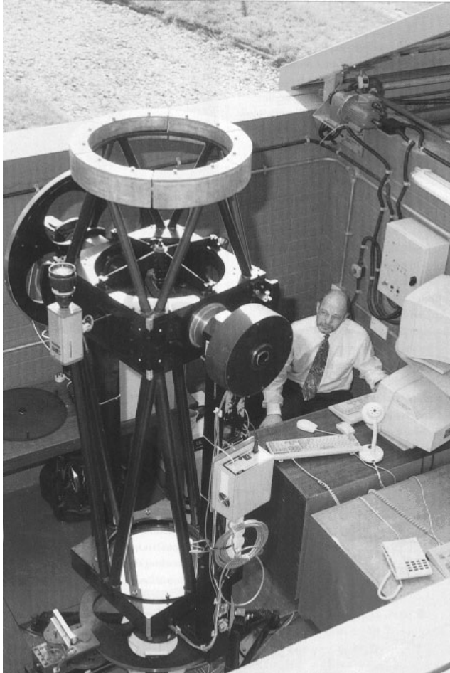
Fig. 6.1.10. John Baruch, director. The University of Bradford's robotic telescope. Scientists and others can direct the telescope's direction of view from anywhere in the world via the World Wide Web, ( http://www.telescope.org/rti/intro.html ).
