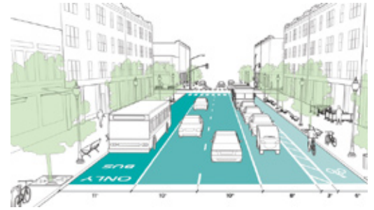
An example of recommended lane widths from the NACTO Urban Street Design Guide.
